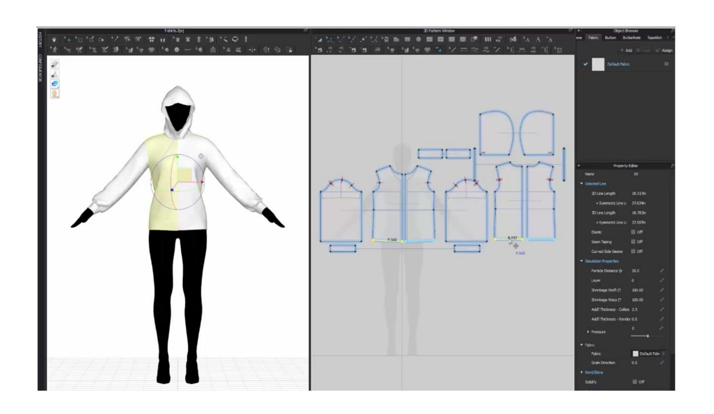
3D pattern design: the interface of a software tools used for making the patterns of a hoodie with the avatar for showing the final result on the side.
